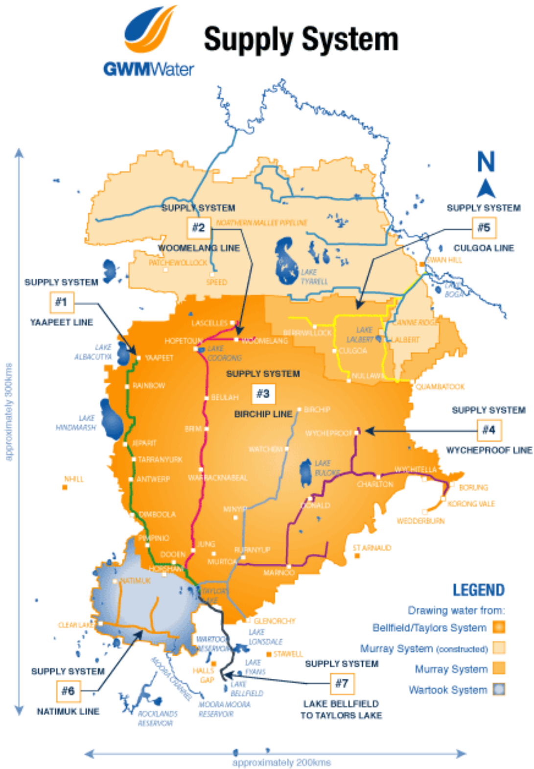
Figure 2- Wimmera Mallee Pipeline Supply System
